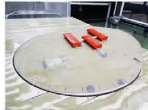
Option 1 model with constant grade topography
